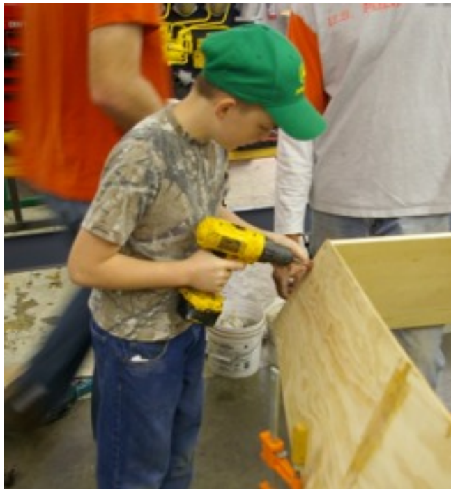
4-H'r Michael Stewart fastening side panel to transom of boat. Photo by Dave Machen
